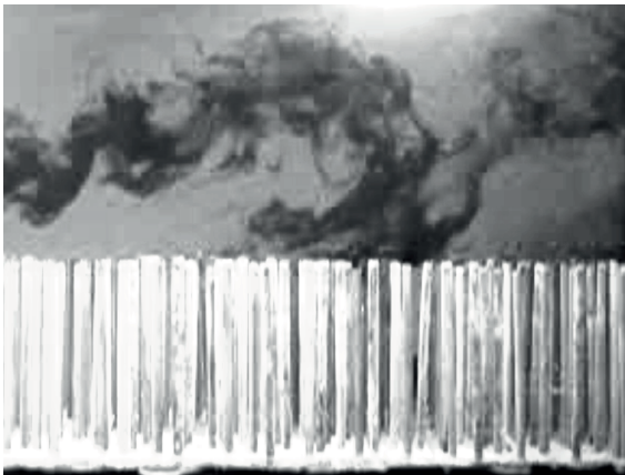
Figure 1: Vortex instability, as indicated by a dye streak, in unidirectional laboratory flow over an array of cylinders (from [7]). The mean flow is from left to right.
